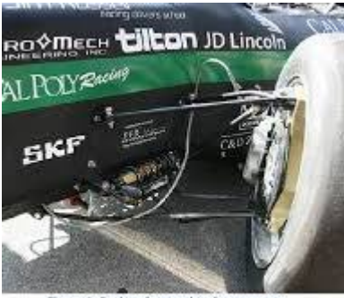
Figure 1: Broken Suspension Components
