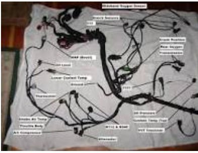
Figure The 1.8T Wiring Harness Explained
